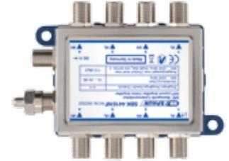
If the terminating resistor in mounted (**This is the delivery status!**), the 12V on the vertical low IF line will be switched off and the unit will work as 4 way inline Amplifier with DC pass and DiSEqC through.
